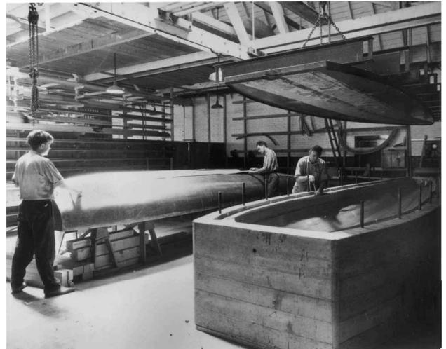
**Fig. 7** Forming Lockheed monocoque fuselage shells in concrete molds (SI negative number 91-3446).
